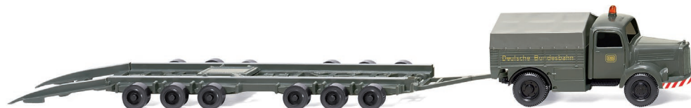
0590 03 Wagon-carrying road trailer Culemeyer (MB L 3500) New heavy load flatbed with tarpaulin 1951-55
